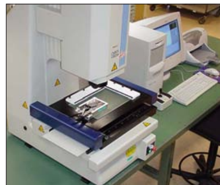
Production station for measuring crimp die nest heights.
