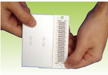
The printed module can be separated using the SI2K009 item
